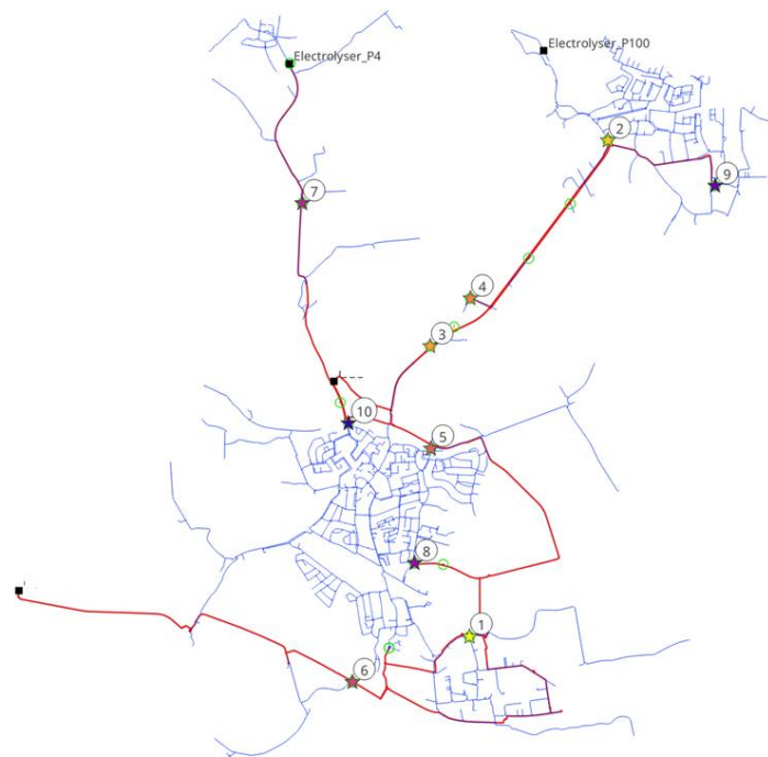
Figure 15: Example output of Aurora gas network simulator from the work done in [4]. The different colours of pipelines indicate different pressure levels. The stars indicate the location of sensors placed by the optimal sensor placement algorithm based on hundreds of random demand scenarios in the network.
