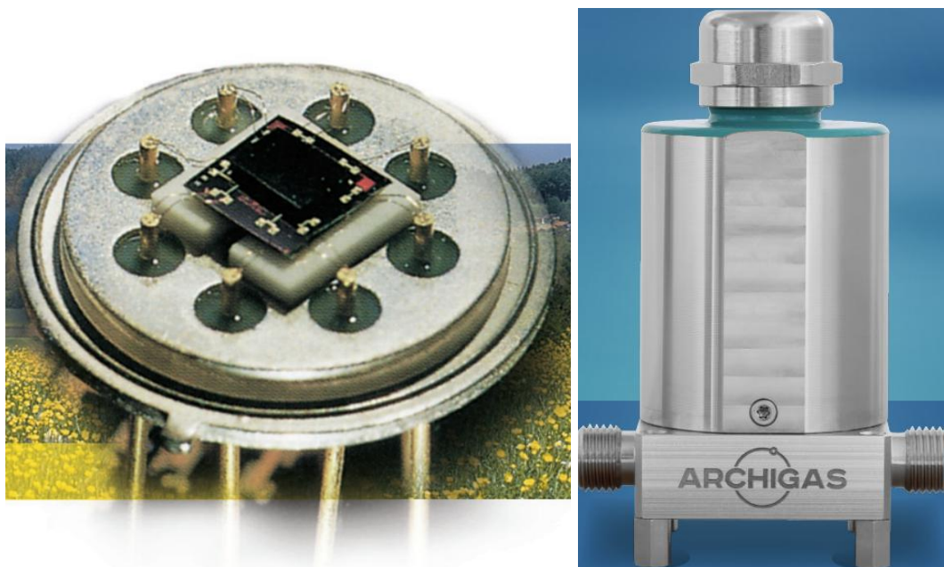
Figure 11: Left: example of a miniature TCD detector [28]. Right: example of an integrated TCD instrument [29].
