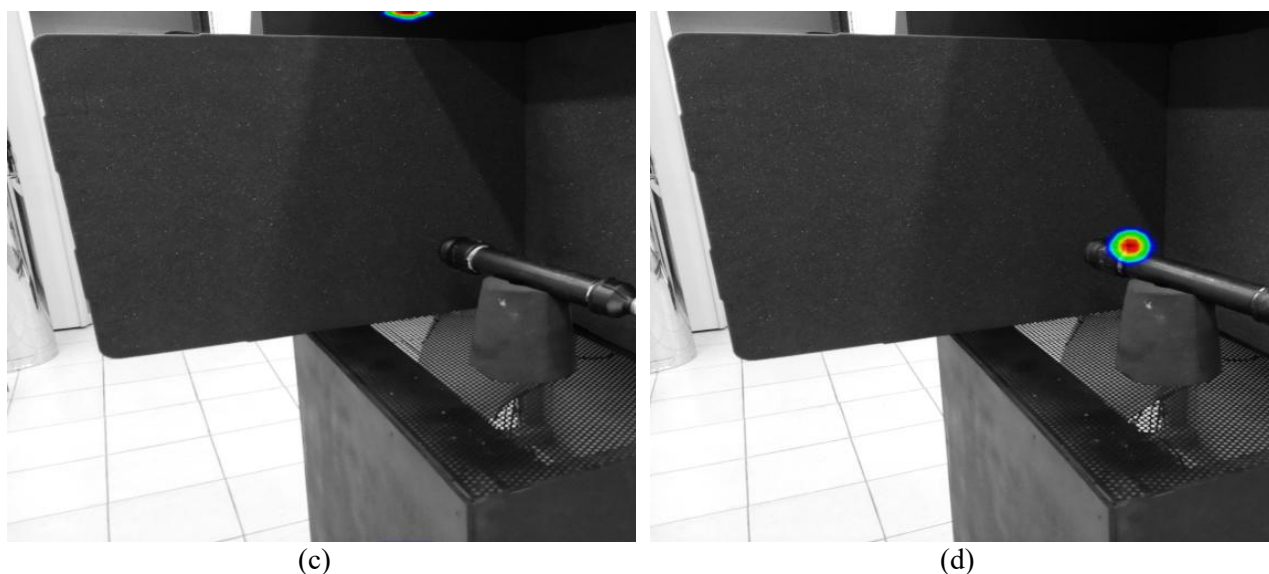
Figure 3-5: Leak detection using acoustic method, leakage at the threaded connections measured for a mixture of natural gas with 20% hydrogen; (a) Camera 1: leak 0.4 l/min, detection; (b) Camera 1: leak 0.8 l/min, detection; (c) Camera 2: leak 0.4 l/min, no detection; (d) Camera 2: leak 0.8 l/min, detection
