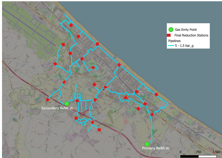
Figure 3-1: higher-pressure level of the natural gas distribution infrastructure of Riccione (INRETE) considered in this deliverable.
