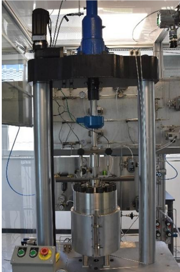
Figure 15 Test machine for SSRT, fracture toughness, and fatigue testing in compressed hydrogen.
