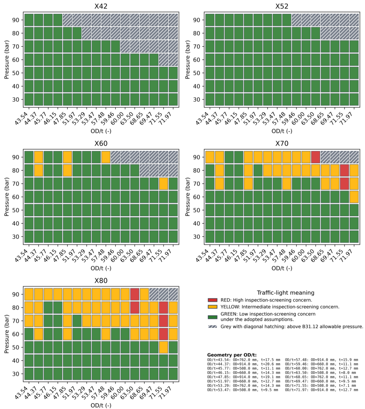
Figure 11. Case-level inspection-screening priorities in 100% H 2 for the large-diameter pipeline matrix. Grey diagonal hatching identifies combinations exceeding ASME B31.12 design conditions.
