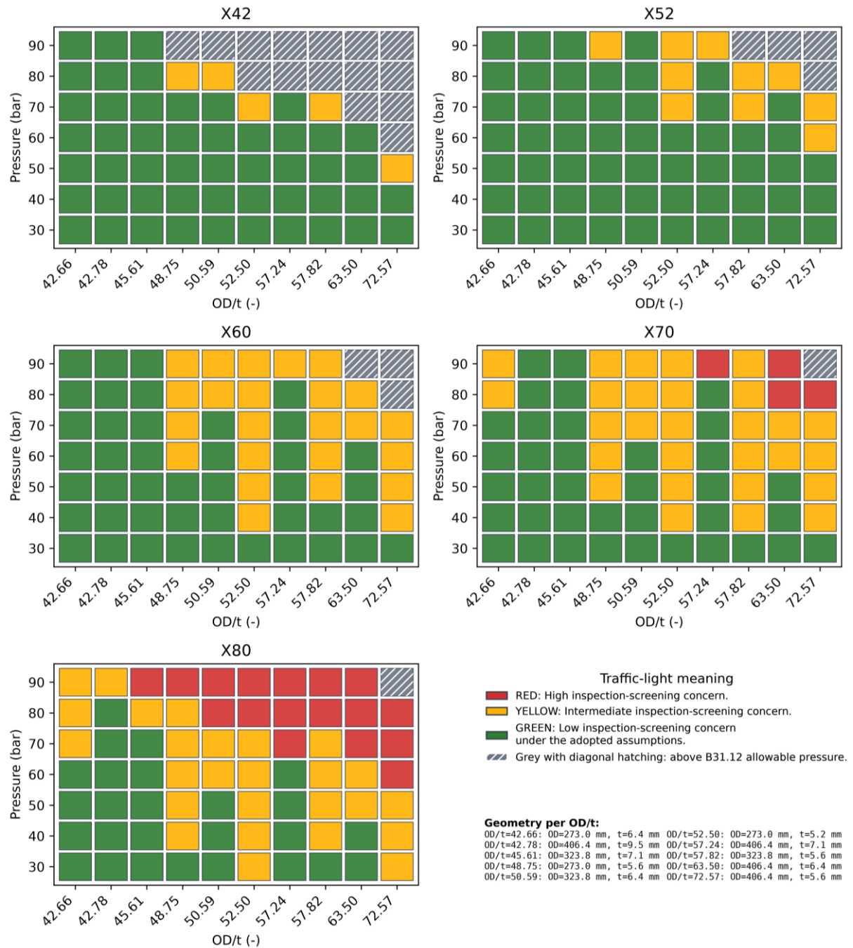
Figure 10. Case-level inspection-screening priorities in 100% H 2 for the medium-diameter pipeline matrix. Grey diagonal hatching identifies combinations exceeding ASME B31.12 design conditions.
